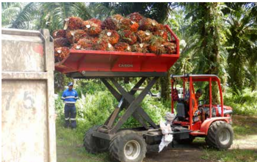
/// Crop transporter with scissor-lift used to collect fruits from inside the field ///
