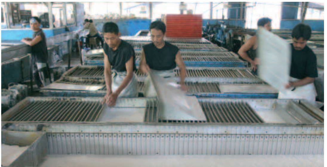
latex coagulating troughs
