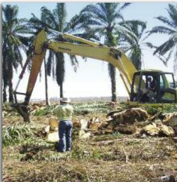
Mechanical shredding of palm trees – zero burning
